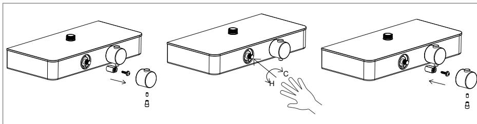
Re-setting thermostatic unit to 38°C starting temperature
